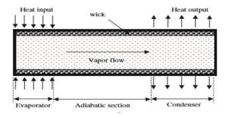
Heat pipe is consisting of three sections are:
